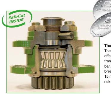
**The innovative, DLG medal awarded and world-first** The SafeCut disc protection system from KRONE offers effective protection and peace of mind. Rather than transferring the shock load of the impact to the cutterbar, the system transfers the load to a roll pin, which breaks as a result of the impact. Then the disc moves 15 mm (0.6") up on its threaded drive pin and out of the risk zone and away from the neighboring discs.
