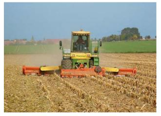
The CM conditioner for 9.0 m (29'6") working widths A flail topper is available as optional specification from our system partner Van Wamel B.V.. The unit will boost machine utilization and effectively fight the corn borer.
