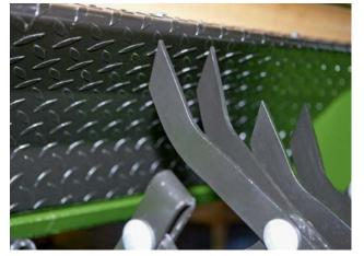
**The CV conditioner for 9.7 m (31'10") working widths** The V-type steel tines on the 66 cm (2'2") diameter rotor feed the crop past a baffle plate to provide intensive conditioning. The operator sets the rotor speed conveniently on the gearbox to 700 rpm or 1,000 rpm and adjusts the baffle plate steplessly.
