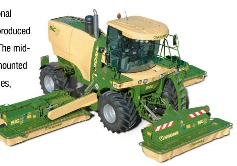
40 km/h (25 mph) as well as a low centre of gravity for ultimate stability on the slope and a direct driveline to the cutterbars. In addition to offering a choice of conditioner versions, BiG M 400 features the unique auger system that merges effectively two swaths into one single swath.
